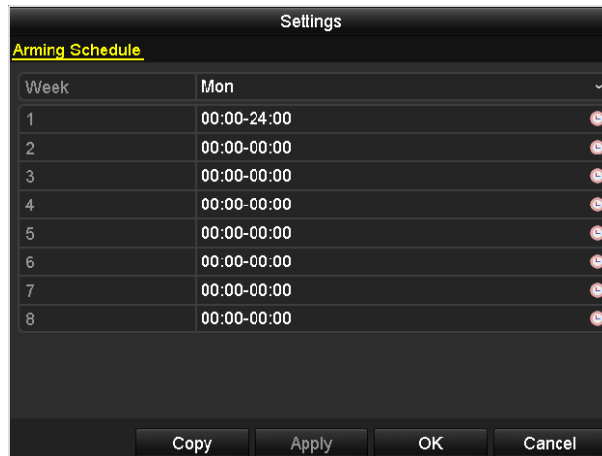
Figure 8-17 Set Arming Schedule of Alarm Output
