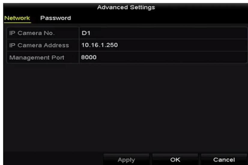
Figure 2-32 Network Configuration of the Camera
