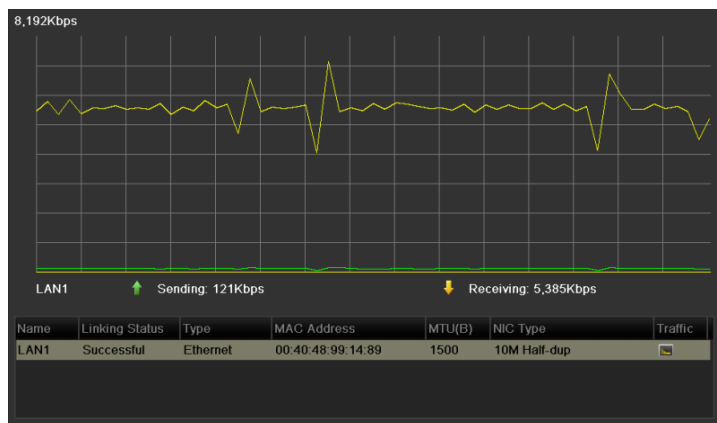
Figure 11-23 Network Traffic Interface
