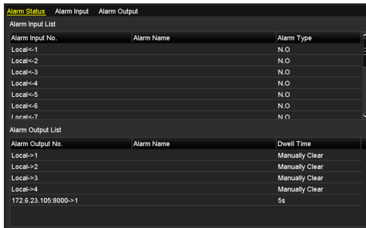
Figure 8-4 Alarm Status Interface of System Configuration
