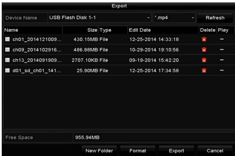
Figure 7-7 Export by Normal Video Search using USB Flash Drive
