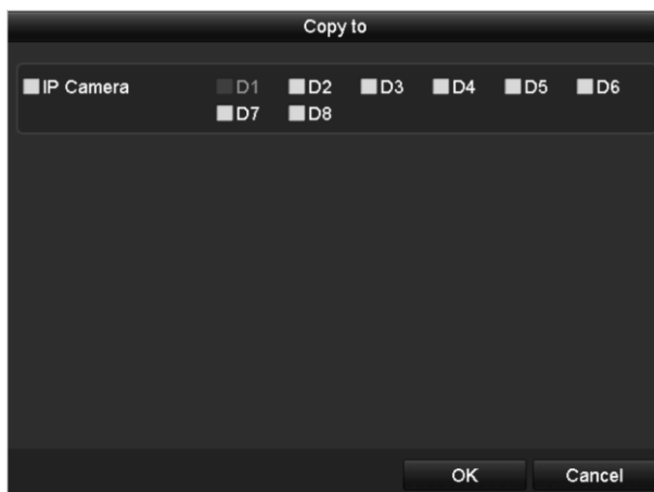
Figure 5-10 Copy Schedule to Other Channels
